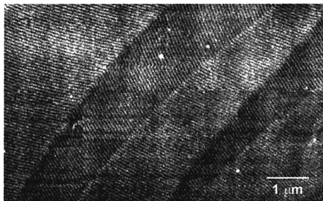
Figure 4. Field emission SEM image of forward kink bands in prealigned SEP(38-62) prior to steady shear. These kink bands, created after steady shear ( 0.005 \text{ s}^{-1} , 80%, half cycle at 180^\circ \text{C} ) and subsequent LAOS, have sharp boundaries, mostly continuous layers across the boundaries with widths of \sim 1 \mu\text{m} . The average angle between matrix lamellae and lamellae within kink bands, \mu , is \sim 40^\circ . Note that the orientation of the lamellae in the matrix near these kink bands is not perfectly parallel and in fact slants downward. Separate images of the starting state show the matrix lamellae near kink bands to be in a variety of orientations (upward, downward, and perfectly parallel). The orientation of the matrix as determined by SAXS is more reliable and is predominately parallel.
